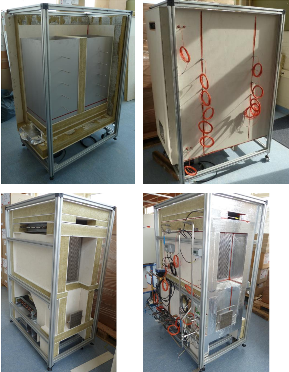
Figure 4-8 pictures of the prototype under construction in the workshop. The upper pictures show the zeolite storage reactors under construction, the pictures below show the air handling unit
