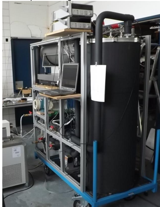
Figure 5-5. The fully built E-hub laboratory fixed-bed zeolite vacuum thermochemical storage set-up, including water baths and monitoring equipment.
