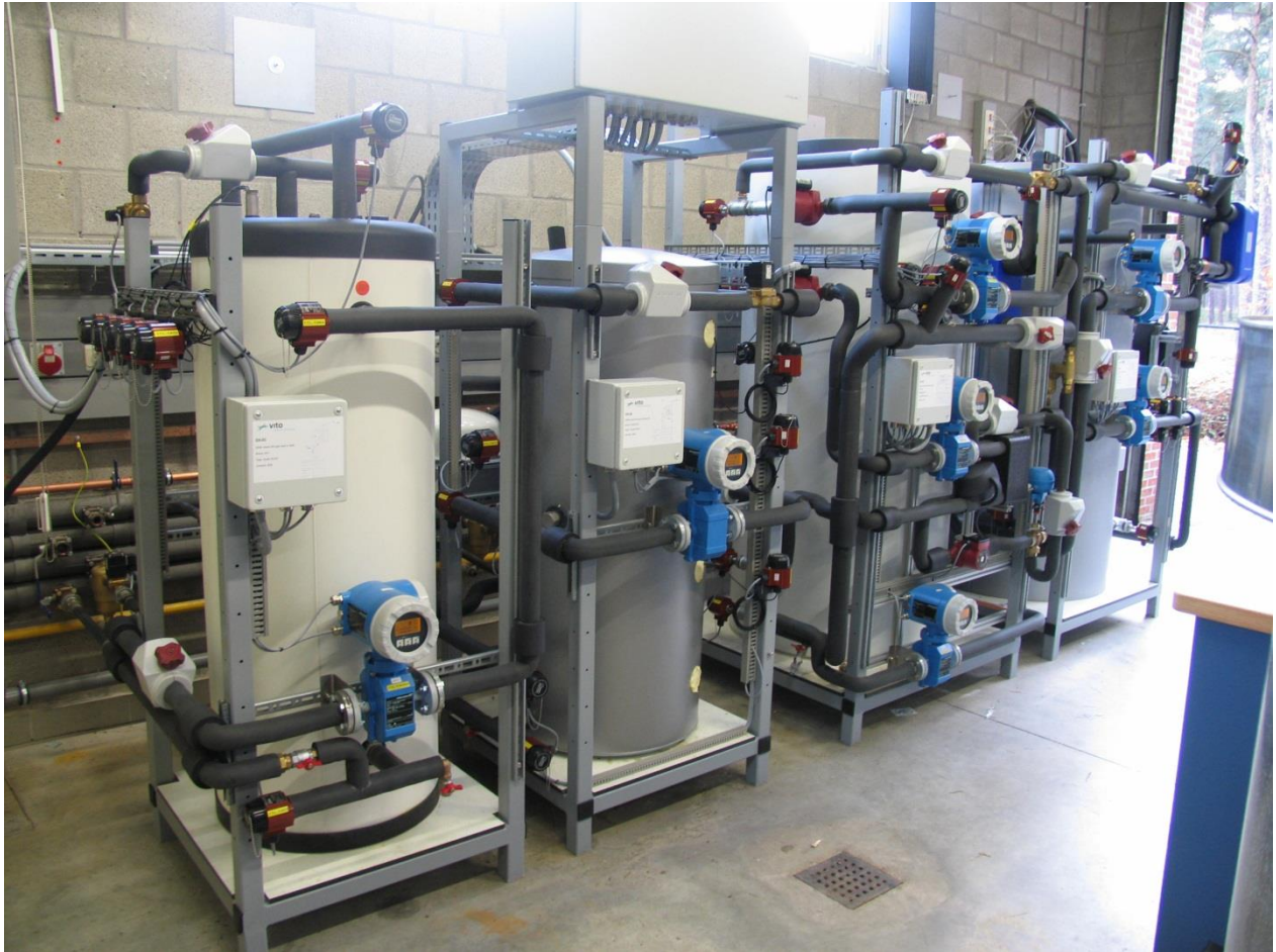
Figure 3-6: Photo of the test setup of the four buffers in the lab of VITO
