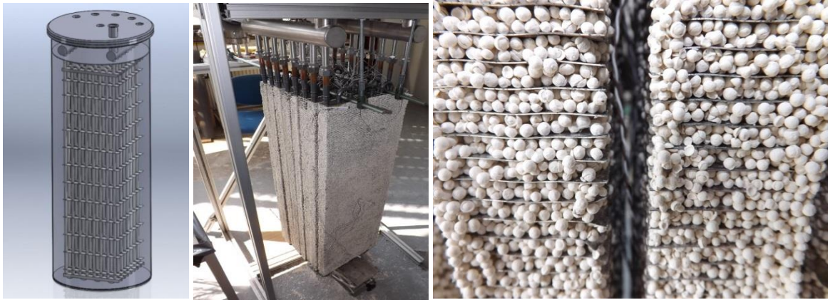
Figure 5-3. Adsorber/desorber finned-plate heat exchangers; (left) 8 adsorber/desorber units containing a total of 41 kg of zeolite spheres during design phase, fitted in a cylindrical vessel; (middle) 8 units during building, before mounting in the vessel; (right) detail.
