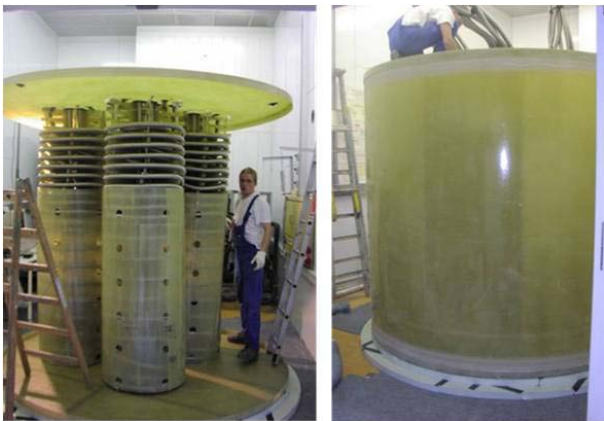
Fig. 43: Glass fiber reinforced plastic (GRP) tanks of company Haase (source: Haase GFK-Technik GmbH)
