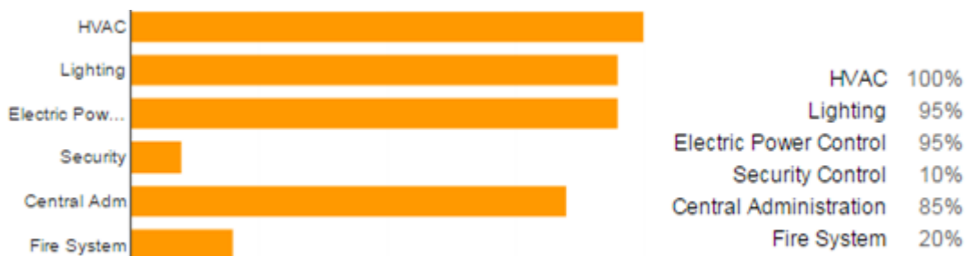
Figure 37 Systems controlled or monitored by the BMS
