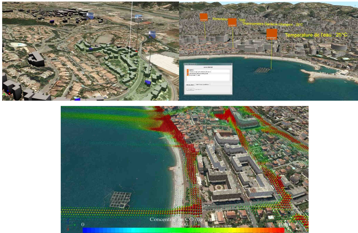
Figure 40 - Some eveCity ways to represent meta and attribute information within a 3D model
