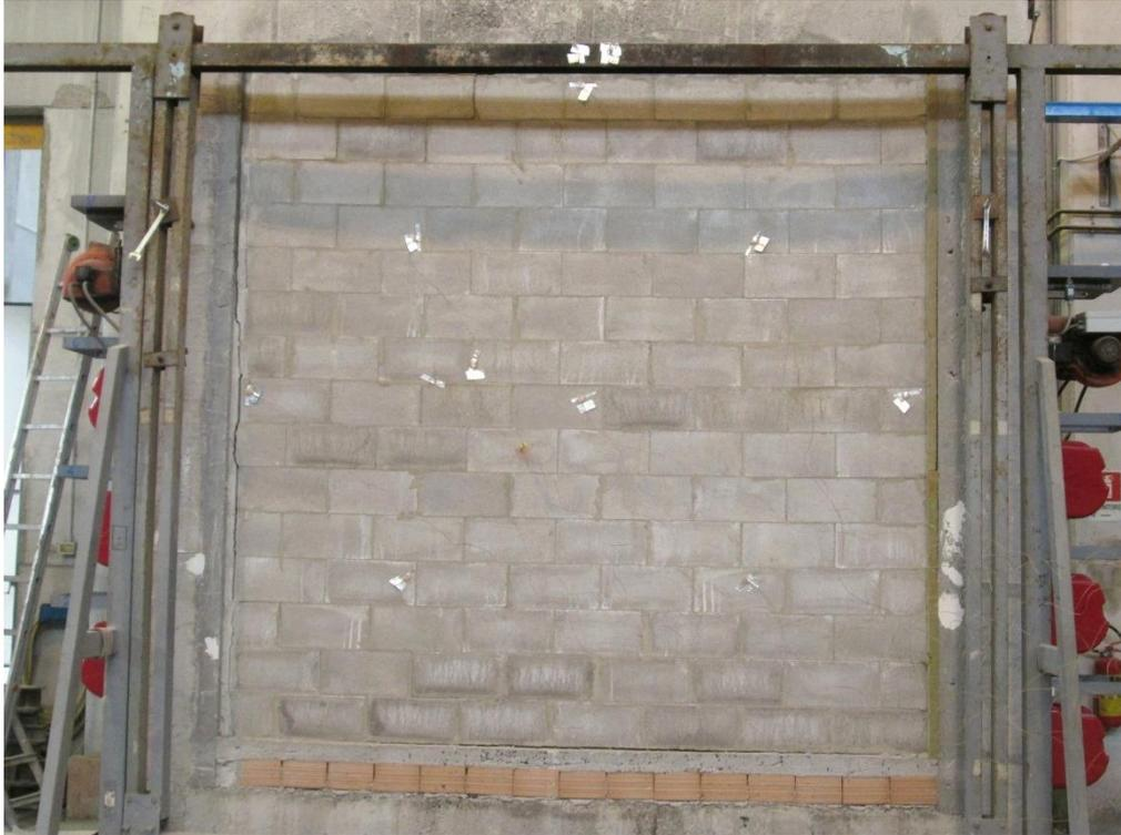
**Figure 27.** After-test photo of the specimen's unexposed face.
