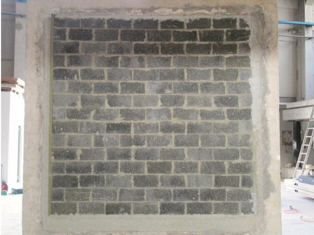
**Figure 29.** Pre-test photo of the specimen's fire-exposed face.
