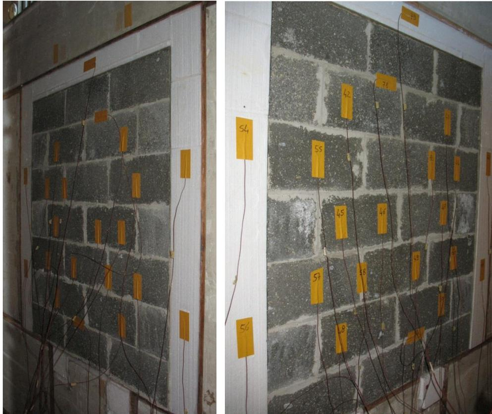
**Figure 8.** Test setup: hot side and cold side.
