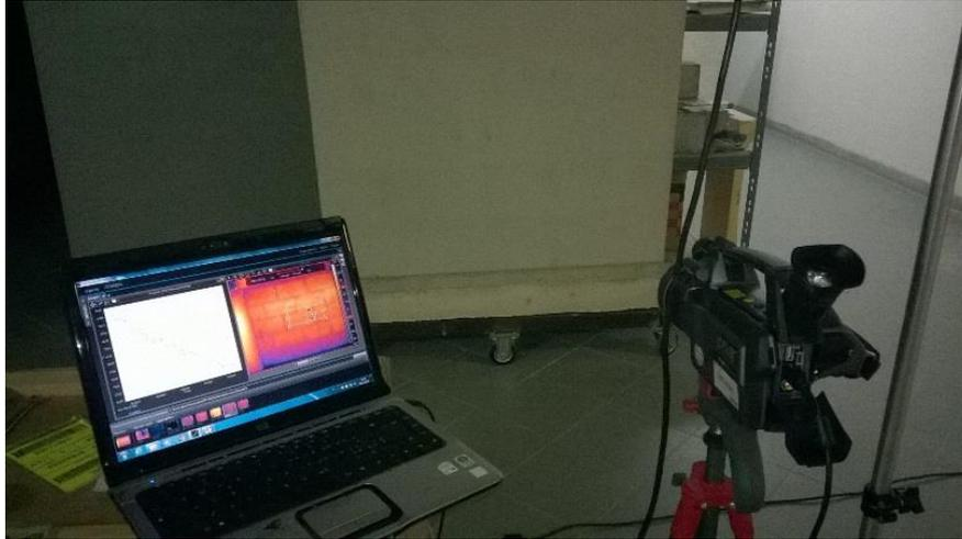
**Figure 45.** Thermographic equipment and software used during the test.
