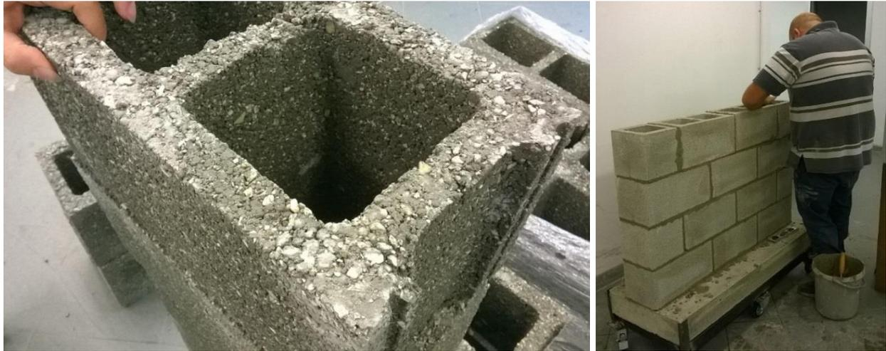
**Figure 42.** SUS-CON Innovative block (left) and SUS-CON Reference block during assembly (right).
