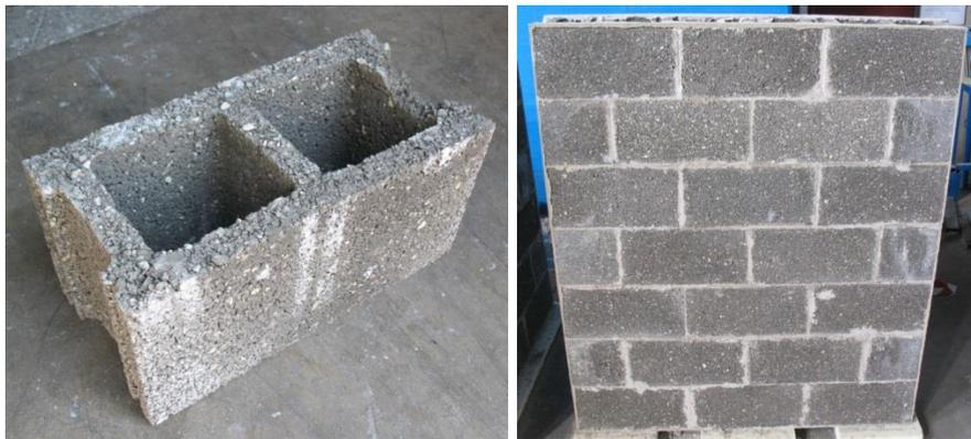
**Figure 6.** SUS-CON masonry unit and wall built for testing.
