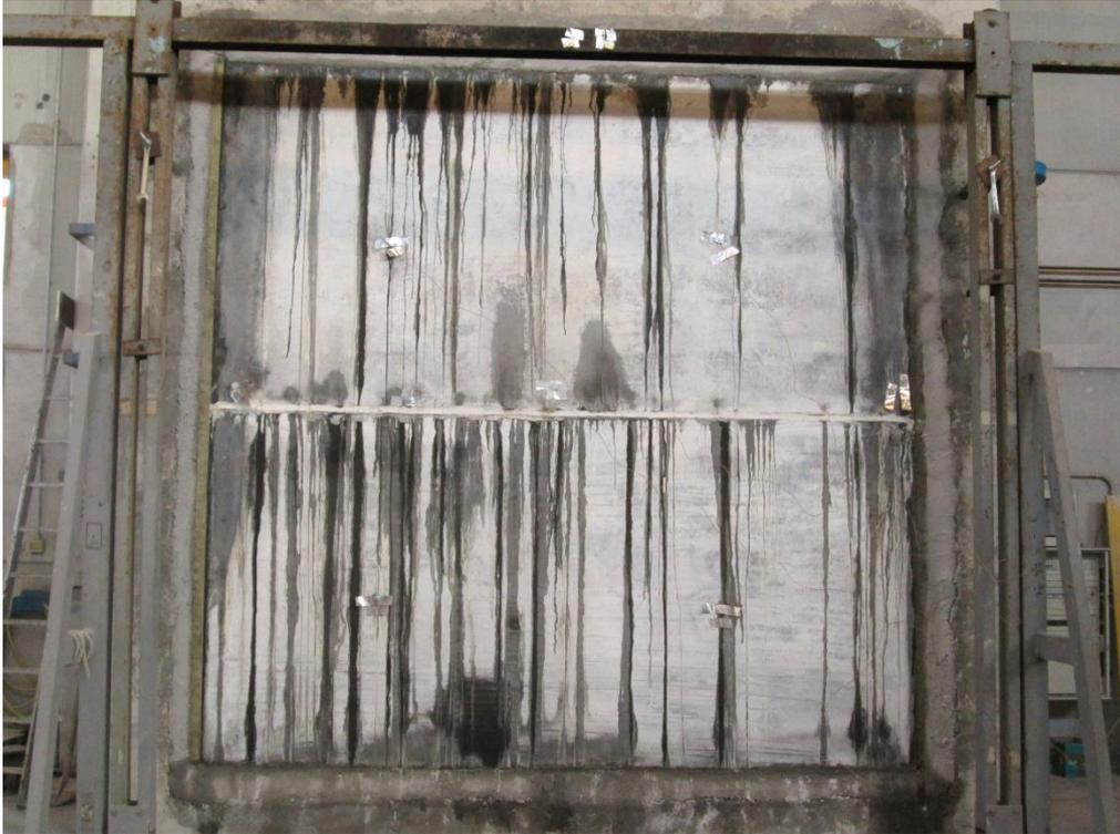
**Figure 41.** After-test photo of the specimen's unexposed face.
