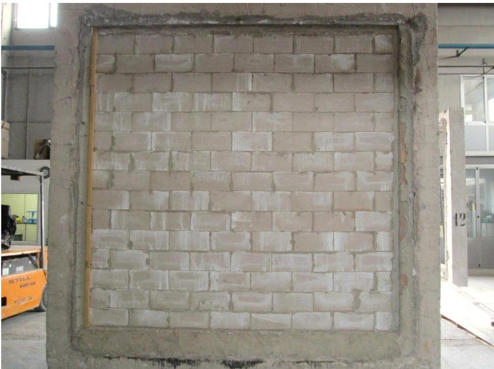
**Figure 26.** After-test photo of the specimen's fire-exposed face.
