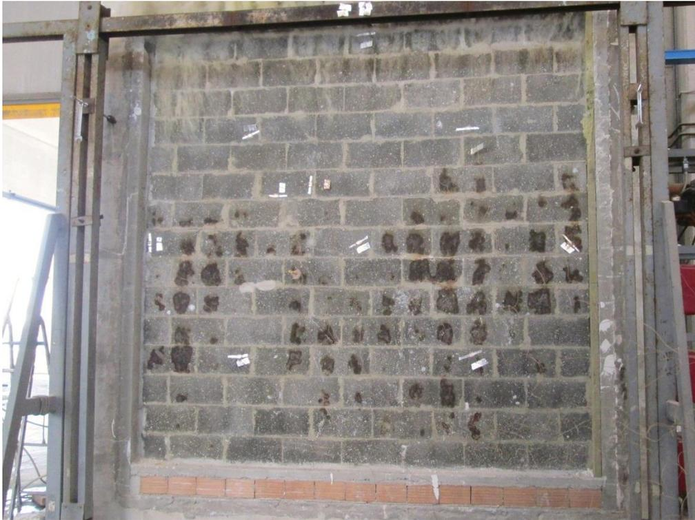
**Figure 31.** After-test photo of the specimen's unexposed face.
