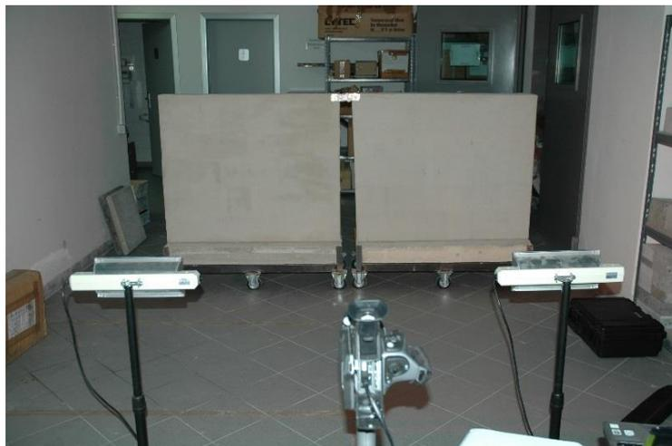
**Figure 44.** W-SIB (left) and W-SRB (right) walls before the thermographic test.
