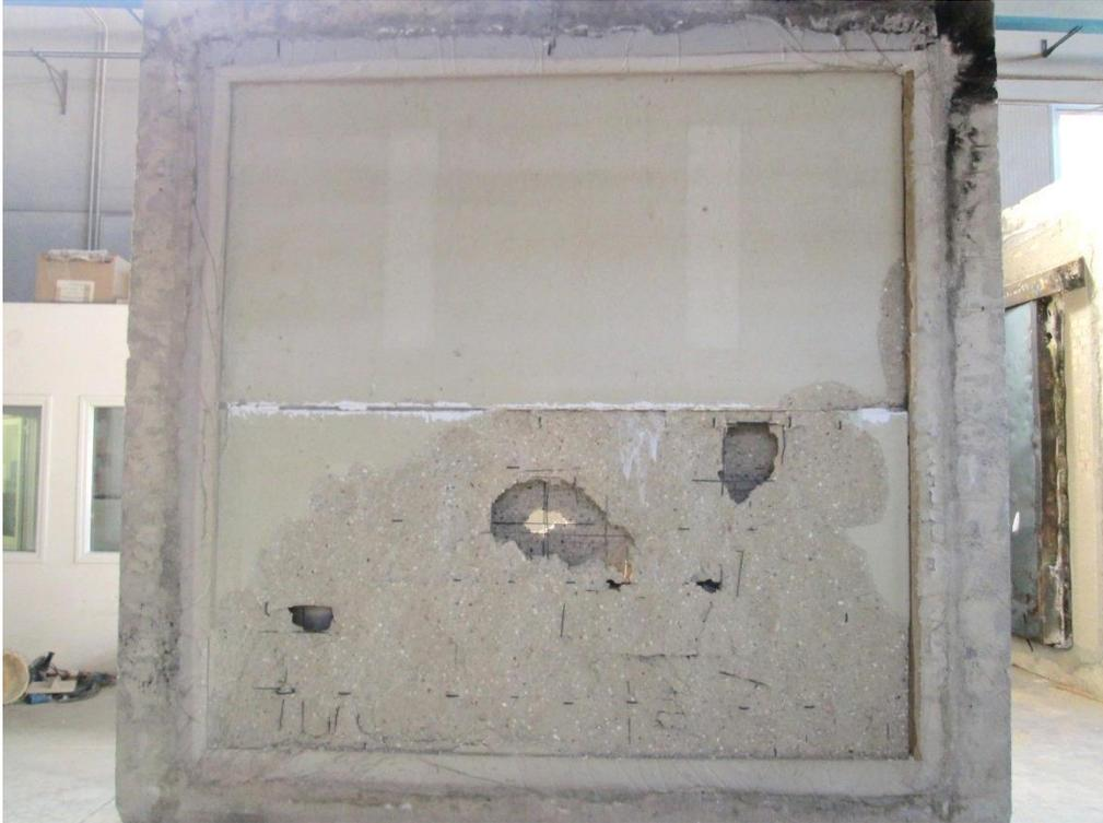
**Figure 36.** After-test photo of the specimen's fire-exposed face.
