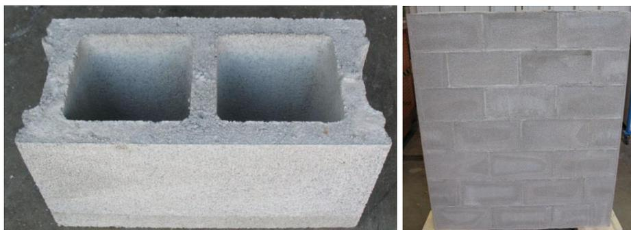
**Figure 7.** REFERENCE masonry unit and wall built for testing.
