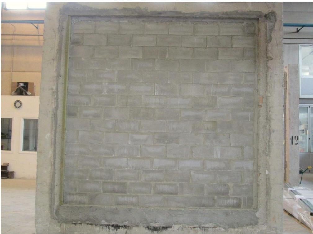
**Figure 24.** Pre-test photo of the specimen's fire-exposed face.
