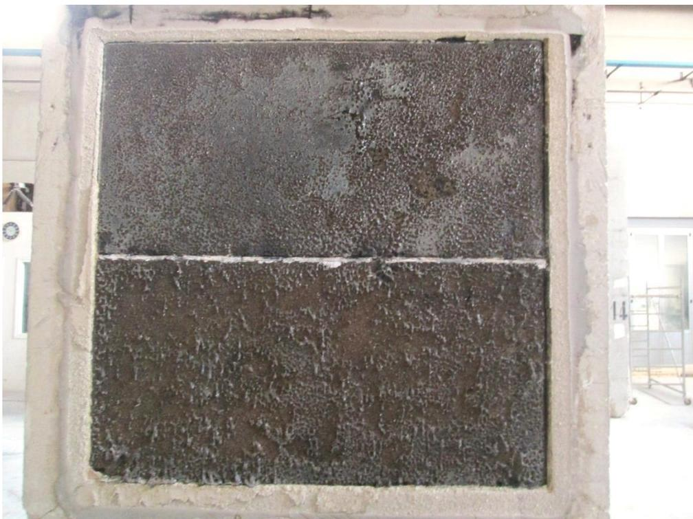
**Figure 40.** After-test photo of the specimen's fire-exposed face.
