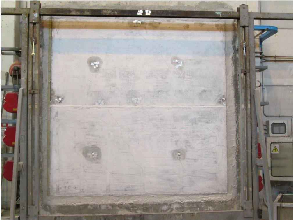
**Figure 39.** Pre-test photo of the specimen's unexposed face.
